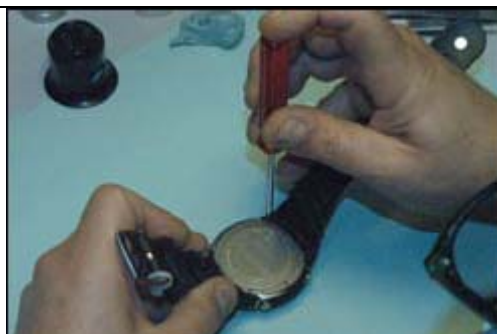
1. Totally unscrew all 5 screws of the case back
