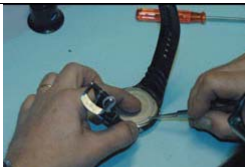
2. Gently remove the screws by using a sharpen tweezers
